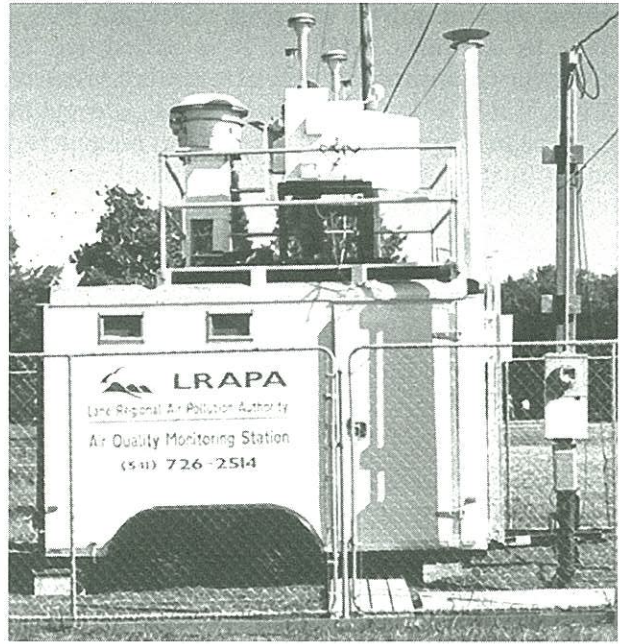
LRAPA monitoring site: one of three sites equipped to collect and log both pollution and meteorological data.
