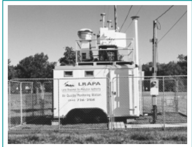
One of three LRAPA monitoring sites equipped to collect and log both pollution and meteorological data.
